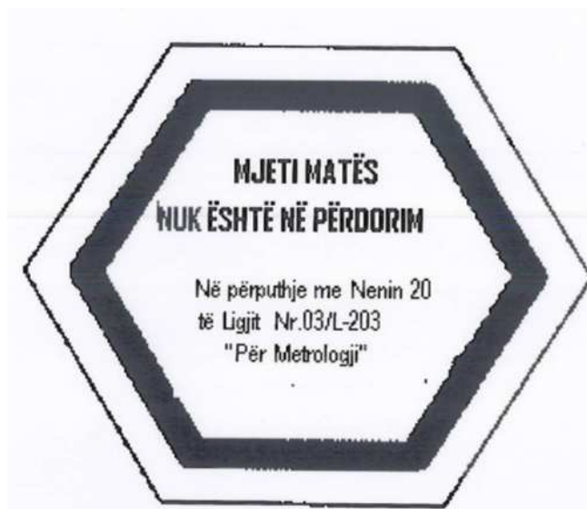
Fig.6.self-sticky paper stamp for marking measuring instruments that are out of use
